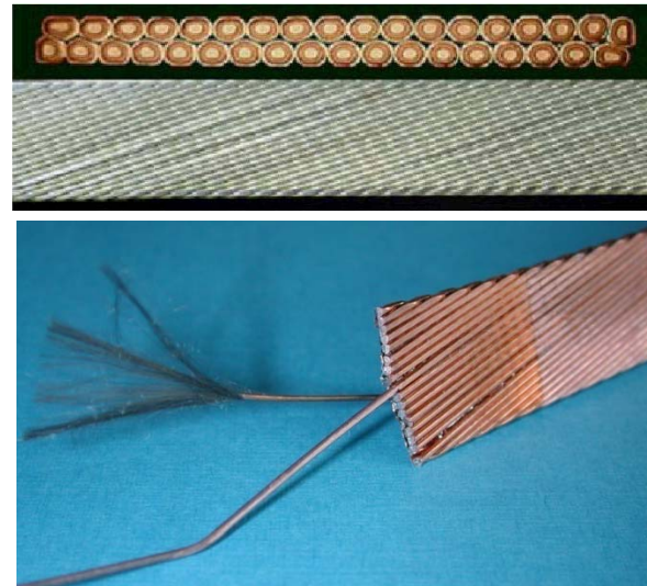
Strands assembled in a Rutherford cable
