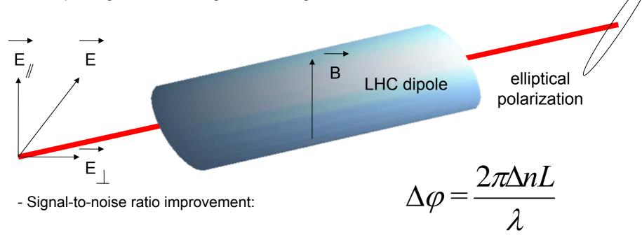
synchronous detection using a linearly polarized laser beam which polarization is rotated at high frequency → unique signature far from low frequency excess noise
