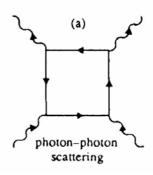
The QED light-on-light scattering produces ellipticity in the linearly polarized light travelling in the magnetic field
