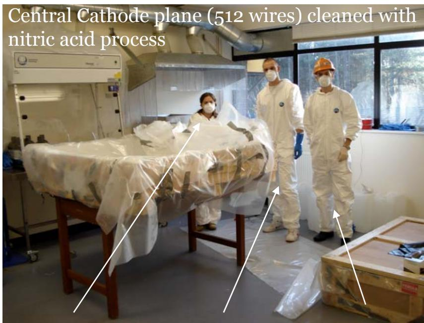
Central Cathode plane (512 wires) cleaned with nitric acid process
