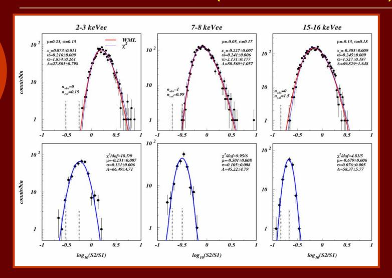
Prediction for ER leakage into WIMP acceptance box: 11.6±3.0 events
