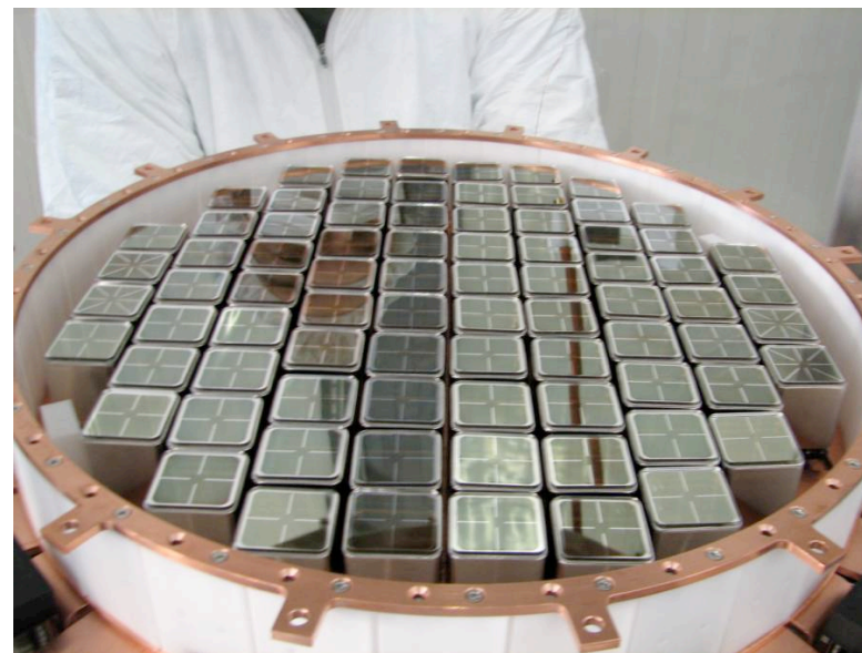
Bottom PMT array (80 PMTs)
